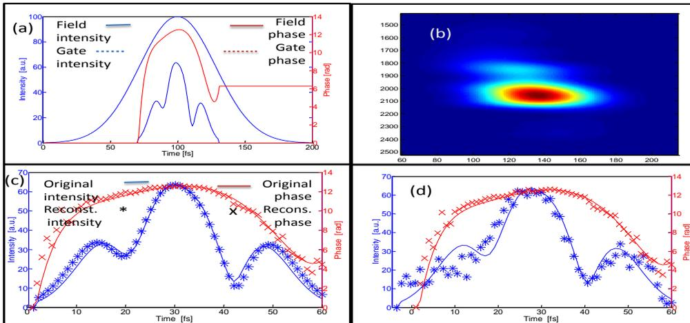
Figure 2: Theoretical super-resolution in cross-correlation frequency resolved optical gating (X-FROG) (a) Amplitudes and phases of the probed and reference pulses (b) calculated spectrogram (c) reconstruction w/o sparsity prior (d) Reconstruction with sparsity prior.
